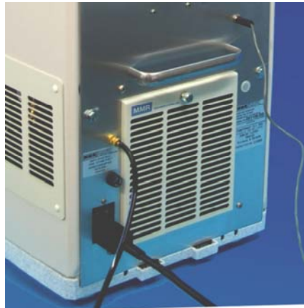
Figure 3. Connections, Power Switch, Fuse, and Air Filter
