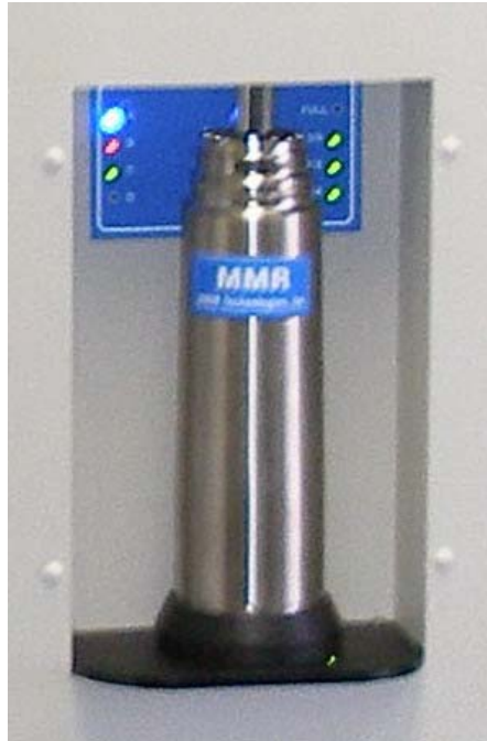
Figure 7. Dewar positioned under chrome spout ready for transfer of LN2.
