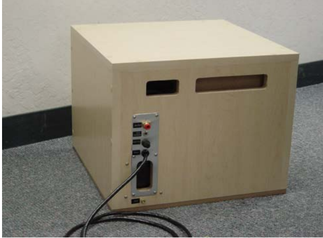
Figure 2. Pressure Swing Absorber and Air Compressor module
