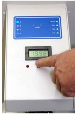
Figure 3. Top view of elan2 AutoTransfer snout showing Display Panel at the top and the Numerical Display (blank) next to the red and green Security LEDs. The volume of LN2 in the external dewar can be seen by pressing the pushbutton on the snout of the elan2-TR just below the Display Panel.
