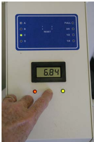
Figure 4. Activate the Numerical Display to show the volume in Liters of LN2 in the external Storage Dewar by pressing the Push-Button between the two Security LEDs.
